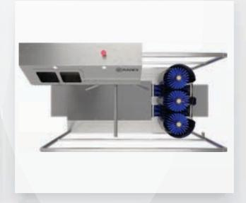
The SHR 05K lock is equipped with a hand disinfection module and rotating brushes for cleaning and disinfecting boots.
