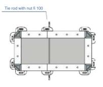
The columns can also be formed from basic formwork using external corners. The above drawings show the examples of this solution.
