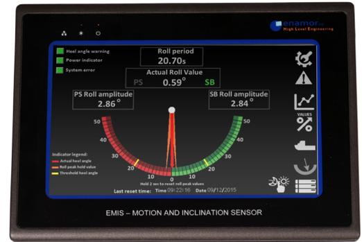
Motion and Inclination Sensor (EMIS) allows measurement of ship motions along her longitudinal (roll) and transverse (pitch) axes. EMIS can be used as stand-alone system with a help of dedicated HMI (Human Machine Interface). Measured signals can be also registered and visualized by parent system (e.g. ESOS for performance analyses). EMIS provides separate roll signal for external systems (e.g. VDR system).
