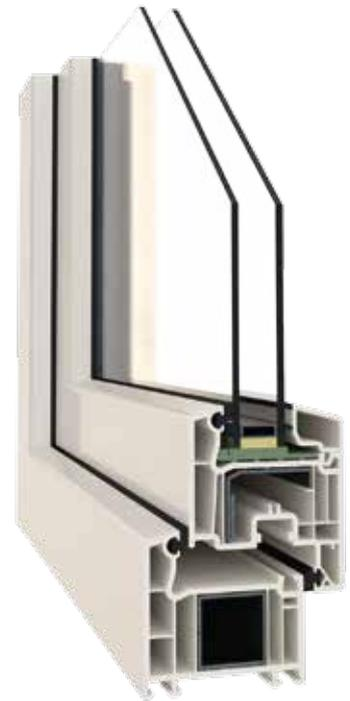
System Perfectline 70 characterized by 5 chambers in the frame and 5 chambers in the sash with an installation profile depth of 70 mm is created to provide heat insulation at a high level. A system of two external gaskets ensures good
