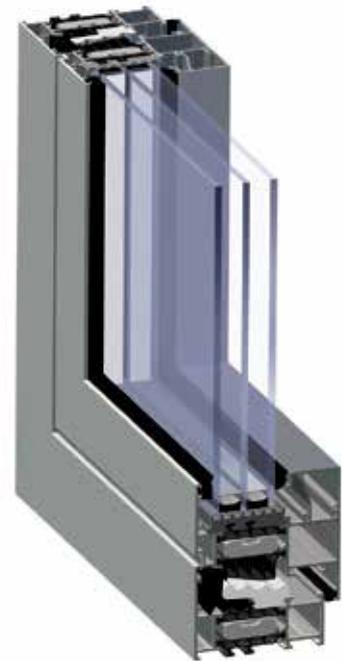
**Genesis** aluminium system designed for windows and doors with increased thermal insulation ( $U_f$  from 0.84  $Wm^2K$ ). This three chambers profile uses modern thermal break solution, which are currently a novelty on the market. Apart from the classic central window gasket, an additional thermal seal was designed, as a result of which a very high tightness was obtained (air infiltration, watertightness) along with an innovative appearance and aesthetics.
